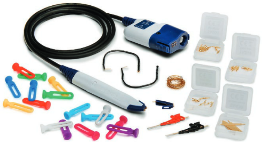
◀ The A3136 1.3GHz Active probes are an optional extra, but are necessary for working at frequencies higher than passive probes can support. The Intelligent Probe Interface powers the probe from the scope and facilitates automatic probe detection and unit scaling.
