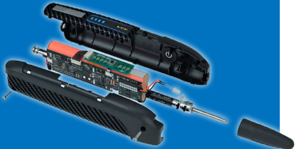
This 3D internal view of the soldering iron showing the battery pack is from the YouTube video: https://youtu.be/0v0tj0m15hA . This same YouTube video also has a 3D external view of the soldering iron.
